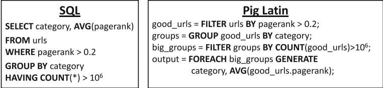
Fig. 9.11 An example SQL query and its equivalent Pig Latin program
